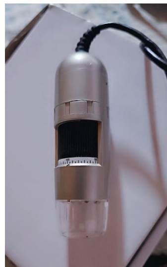
Figure 3. Dino-Lite digital microscope used for examination, documentation, and photography of the collected insects during the study.
